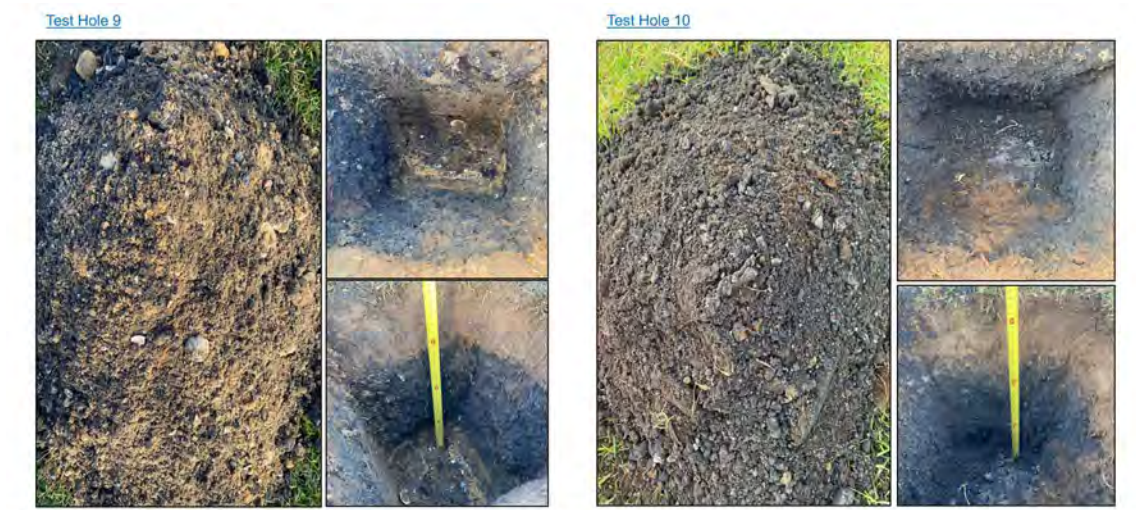
Figure 2: Photographs of ashy fill material encountered at Timbrell Park
