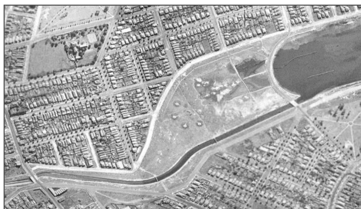
Figure 2.4: The final stages of reclamation of Iron Cove and creation of Timbrell Park – draining and filling behind the sandstone seawall at the head of the bay – in 1942 (Six Maps 2019)
