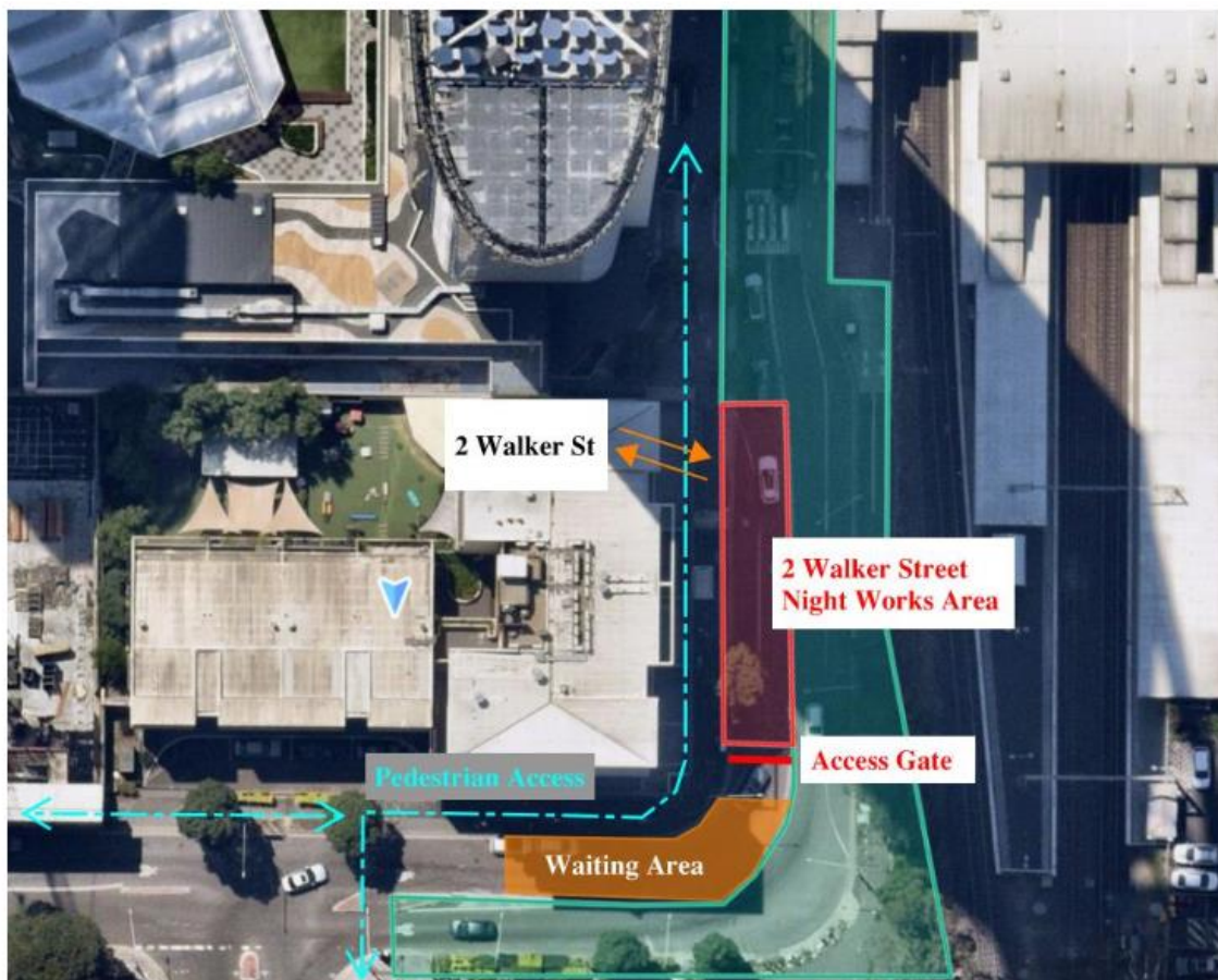
2 Walker St - Night Works Setup
