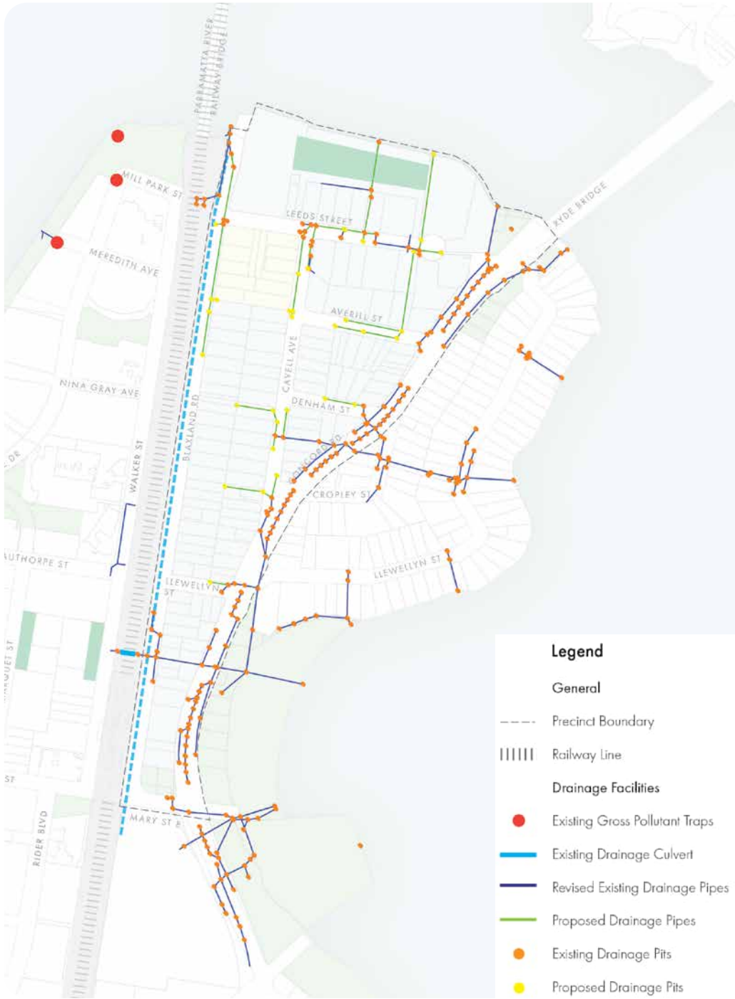
Figure 12. Pits and Pipes Map
